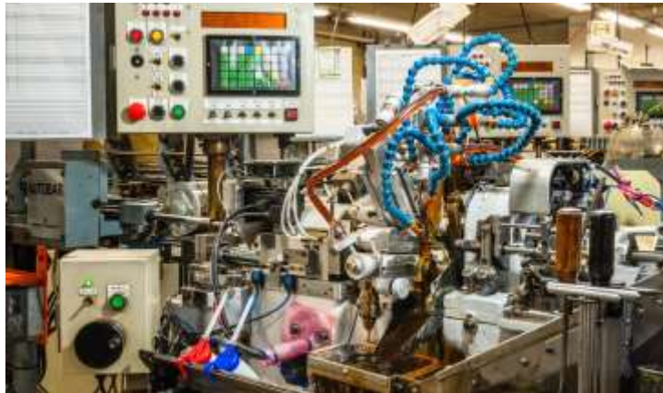
Cam-type automatic lathe Peterman Type 8 (P8)
